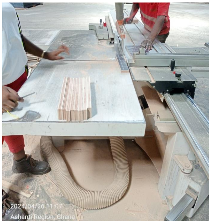
Figure 3: Shows bending samples being prepared using a dimensional saw (MJ320 M Model). (Source: MIRO Timber Products Ltd. Workshop)
