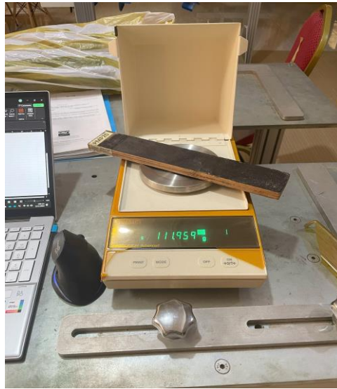
Figure 12: Labelled sample being weighed before drying (Ohaus weighing Scale).
