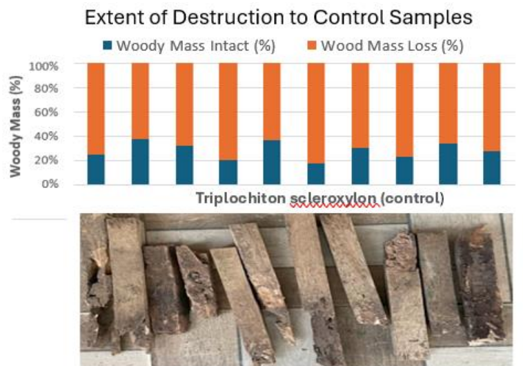
Figure 19: Graph and Image of the control samples after 7 months of exposure to termites
