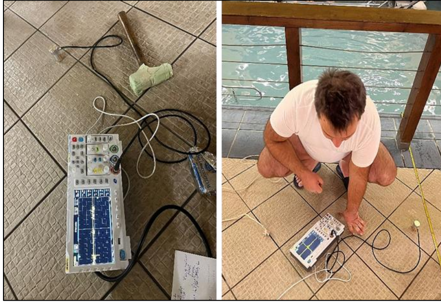
Figure 2.7 Oscilloscope-Based Measurement and Signal Detection Setup for Pile Vibration Analysis (Author).
