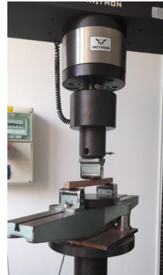
Figure 33: Prepared wood samples and Instron UTM for modulus of rupture and modulus of elasticity.
