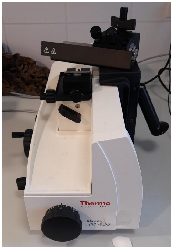
Figure 29: Sliding Microtome for wood sectioning.
