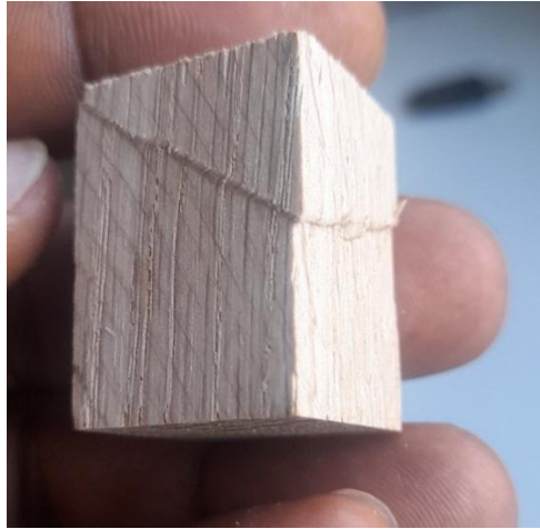
Figure 34: Typical outlook of compressed Turkey oak wood sample.
