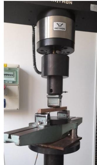
Figure 33: Prepared wood samples and Instron UTM for modulus of rupture and modulus of elasticity.
