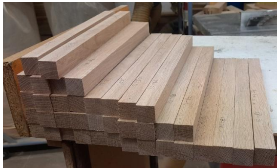
Figure 33: Prepared wood samples and Instron UTM for modulus of rupture and modulus of elasticity.
