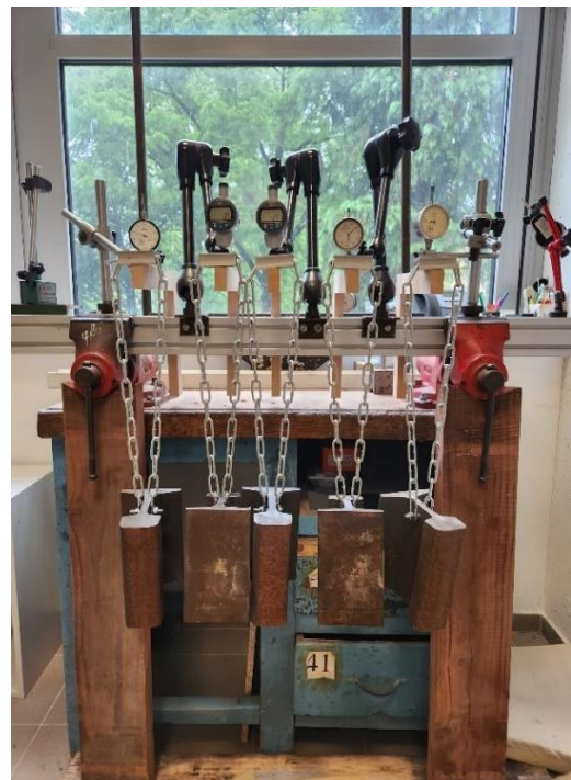
Figure 2.10 Creep test setup for the small test pieces (Photo: S. Baş)
