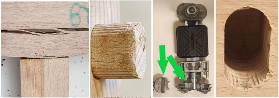
Figure 3.4 Typical deterioration of wood dowels during tension tests (Photo: S. Baş)
