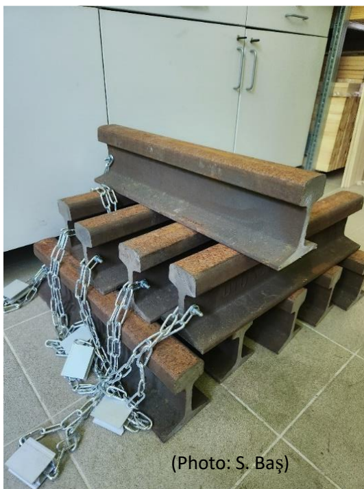
Figure 2.9 Weights used in the creep test for the big test pieces
