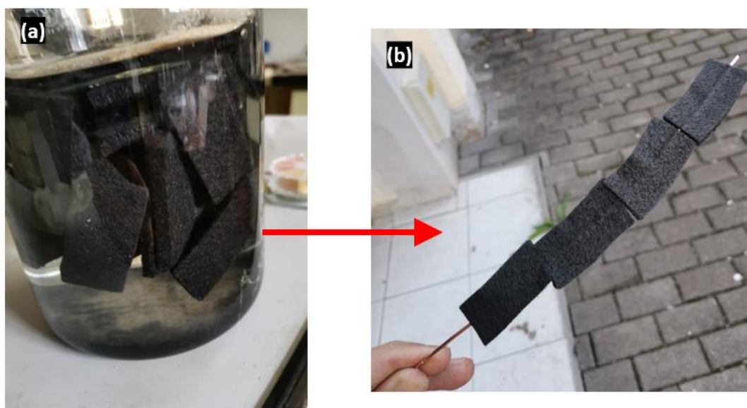
Figure 2.1 The anode electrode preparation. (a) the carbon felt cut and immersed in HCl. (b) four sliced pieces of carbon felt joined through a copper wire.
