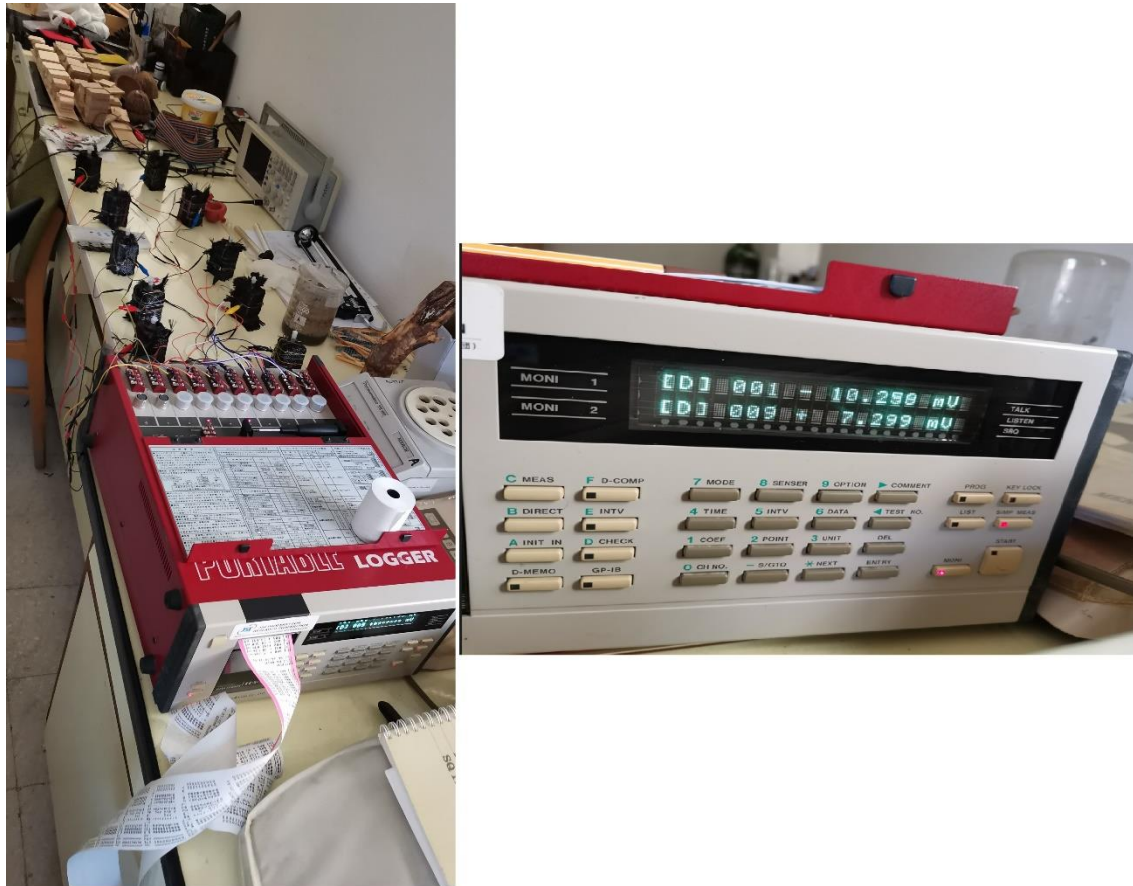
Figure 2.4 TML portable TDS-302 analog data logger for measuring voltage.
