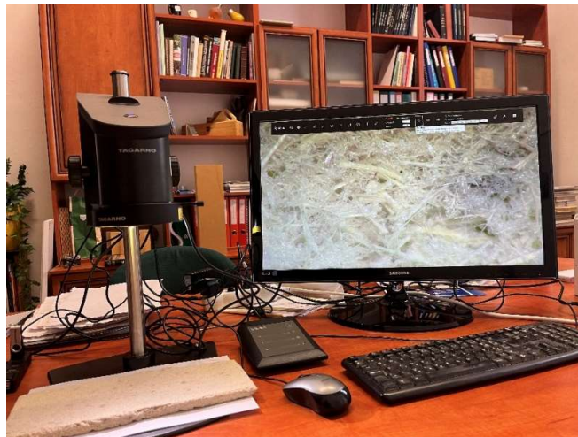
Figure 2.9 Photograph of digital microscope Targano FHD equipment.
