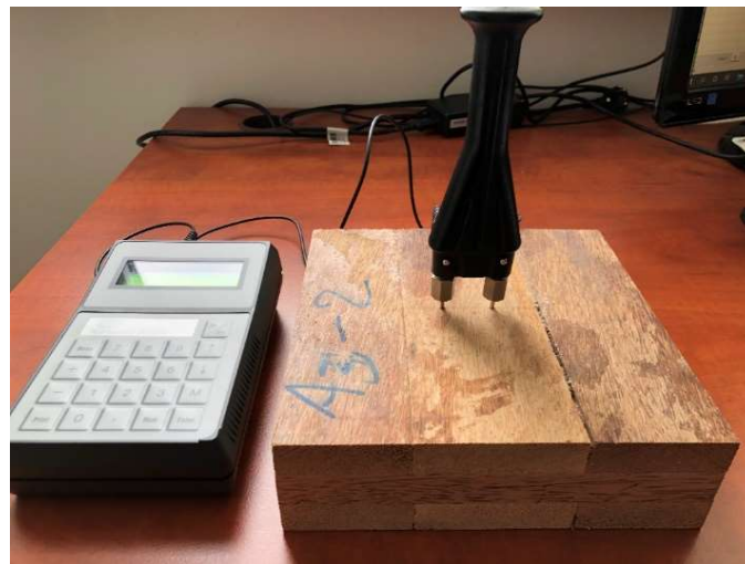
Figure 2.8 Photograph of testing the moisture content percentage of CTCP specimen.
