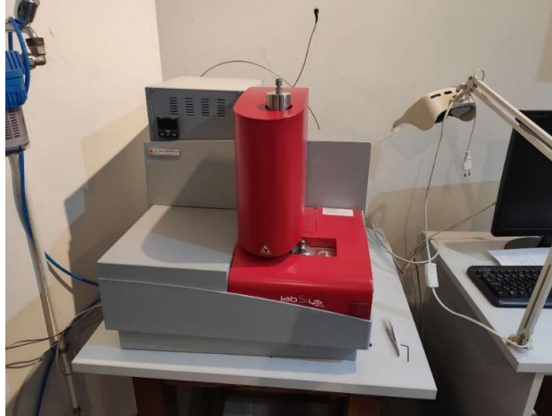
Figure 2.12 Photograph of TGA equipment.
