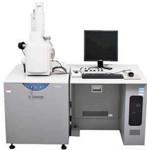
Figure 2.10 Photograph of SEM Hitachi S-3400N equipment.
