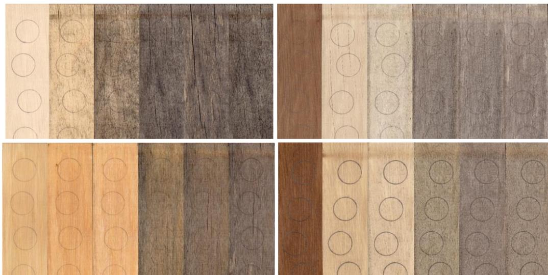
*Figure 48. Series of photos of hornbeam samples exposed to weather. It shows the scans of the untreated (left), acetylated (right), uncoated (up), and coated (bottom) samples before weather exposure, and after 1, 2, 4, 7 and 10 months of weathering (since July 2016).*
