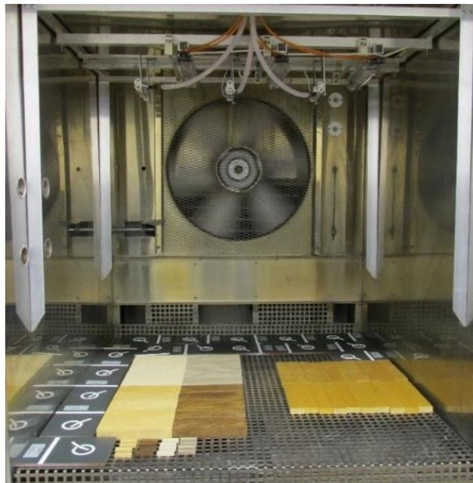
*Figure 33. Uncoated and coated hornbeam and acetylated hornbeam samples placed in the ageing machine with mercury-vapor lamps.*
