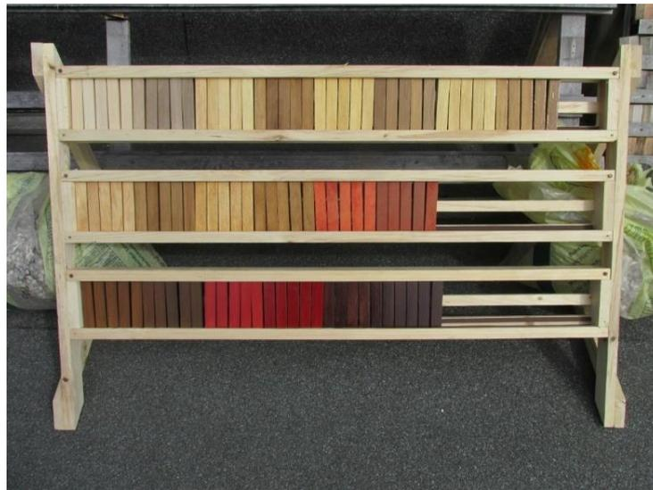
*Figure 49. Weather exposure of untreated and acetylated hornbeam wood coated with various oils and stains.*
