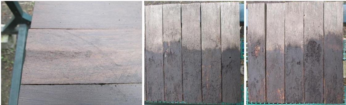
Figure A82. Brown rot in acetylated hornbeam stake no. 7 (left), decayed and insect-damaged untreated hornbeam (middle) and beech stakes (right) after 1.5 years of exposure.
