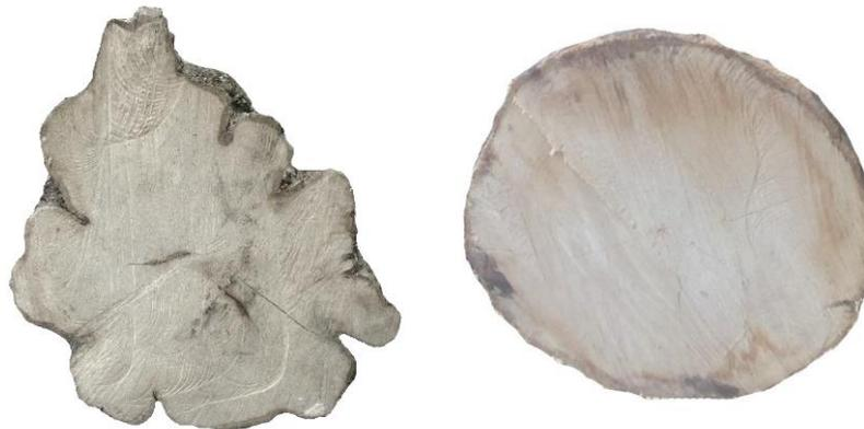
*Figure 6. Disks made from fluted (left) and cylindrical (right) hornbeam logs.*
