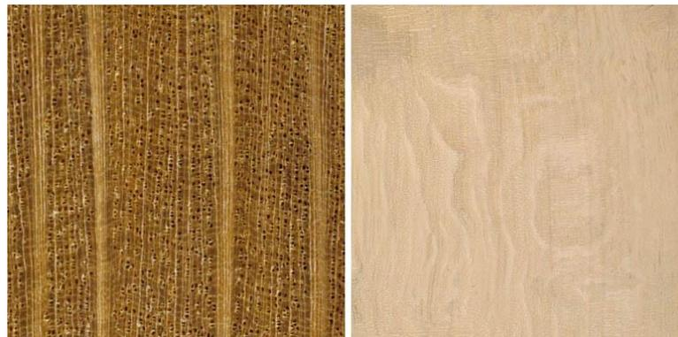
*Figure 7. Transverse section (left, ca. 10x) and radial section (right) of natural hornbeam wood (Richter and Dallwitz, 2019).*
