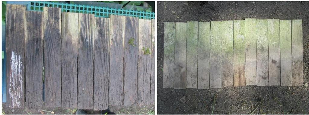
Figure A84. Severely damaged Scots pine stakes after 3.5 years (left), and sound acetylated hornbeam stakes after 4 years of exposure.
