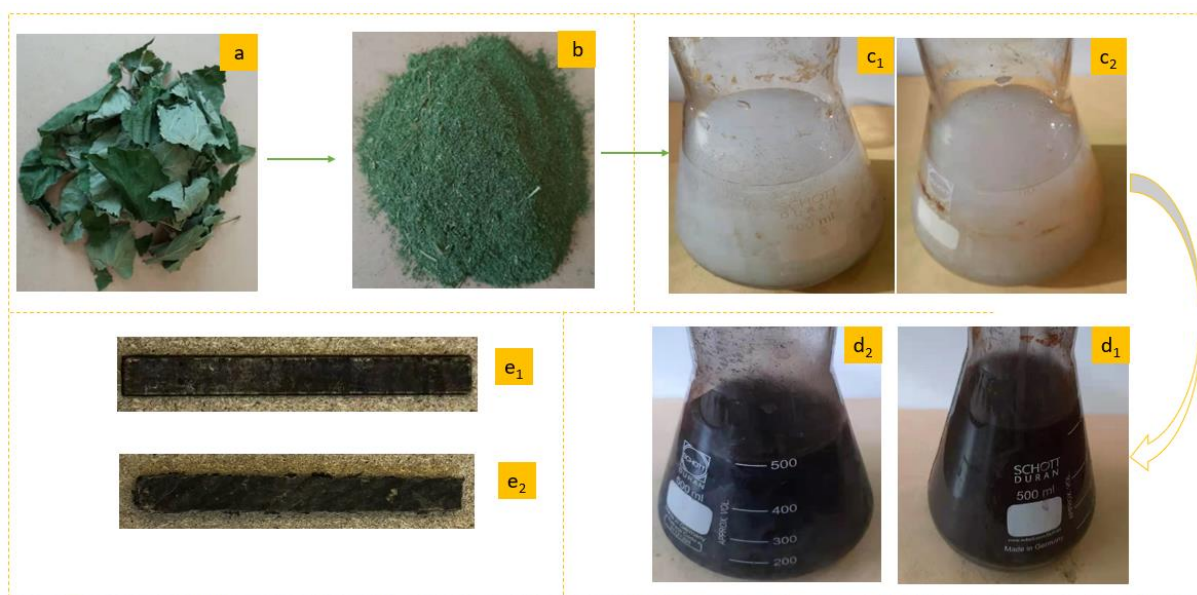
Figure 4.9: Schematic representation of synthesis and application of green AgNPs: (a) dried Tilia cordata leaves; (b) crushed Tilia cordata leaves powder; (c 1 and c 2 ) AgNO 3 precursor in distilled water (1.0 and 5.0 mM concentration, respectively); (d 1 and d 2 ) synthesized green AgNPs solutions for different precursor; (e 1 and e 2 ) bending test species of produced composites from greenly synthesized AgNPs treated woven fabrics.
