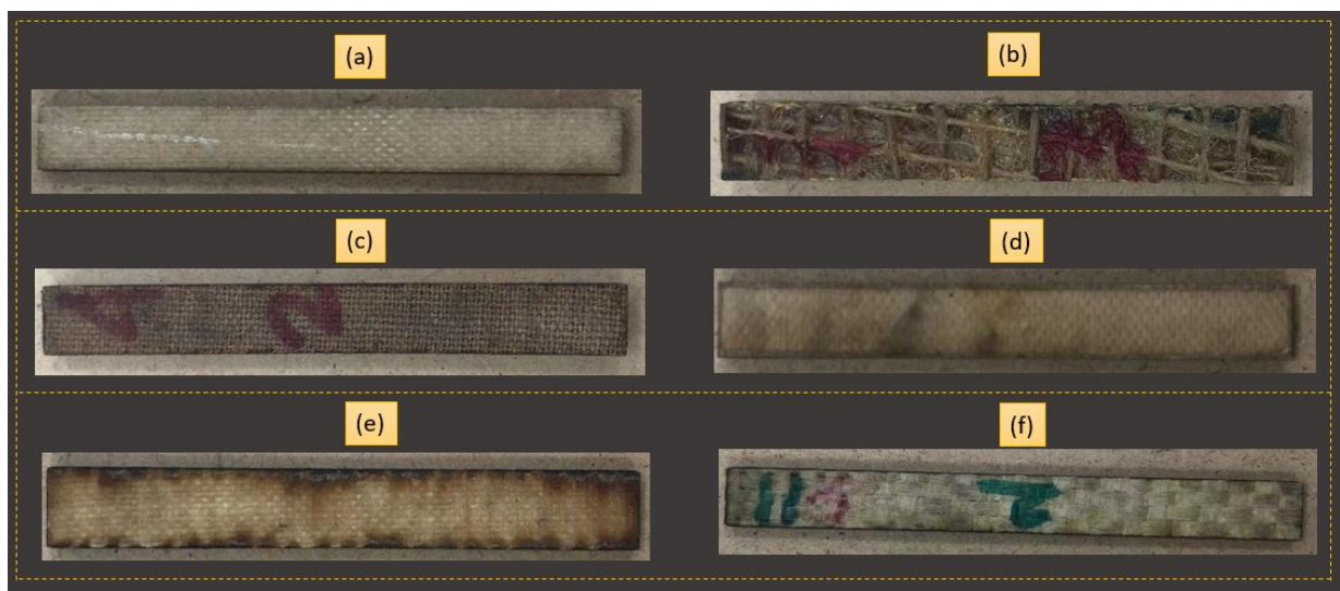
Figure 1.8: Composite samples from different woven fabrics developed in our lab: (a) flax woven fabric reinforced PP composites, (b) jute woven fabric reinforced MDI composites, (c) flax woven fabric reinforced MDI nano composites (AgNP loaded), (d) flax woven fabric reinforced PLA composites, (e) hemp/glass woven fabric reinforced epoxy composites, (a) glass/flax woven fabric reinforced MUF composites.
