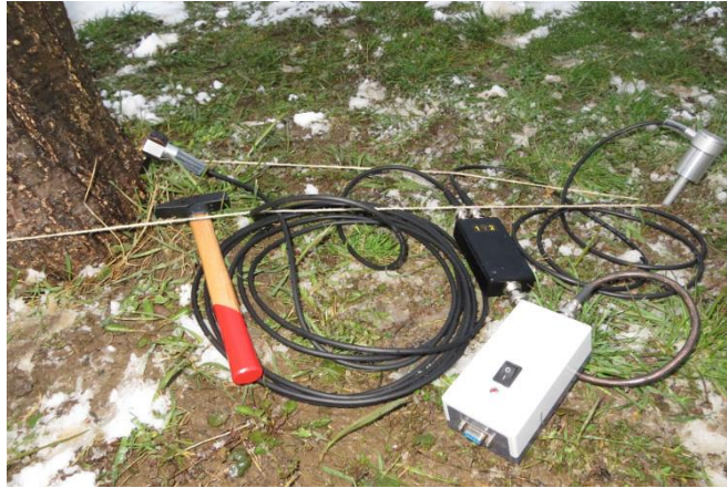
Figure 6 – Photograph showing the measurement principle used for root detection
