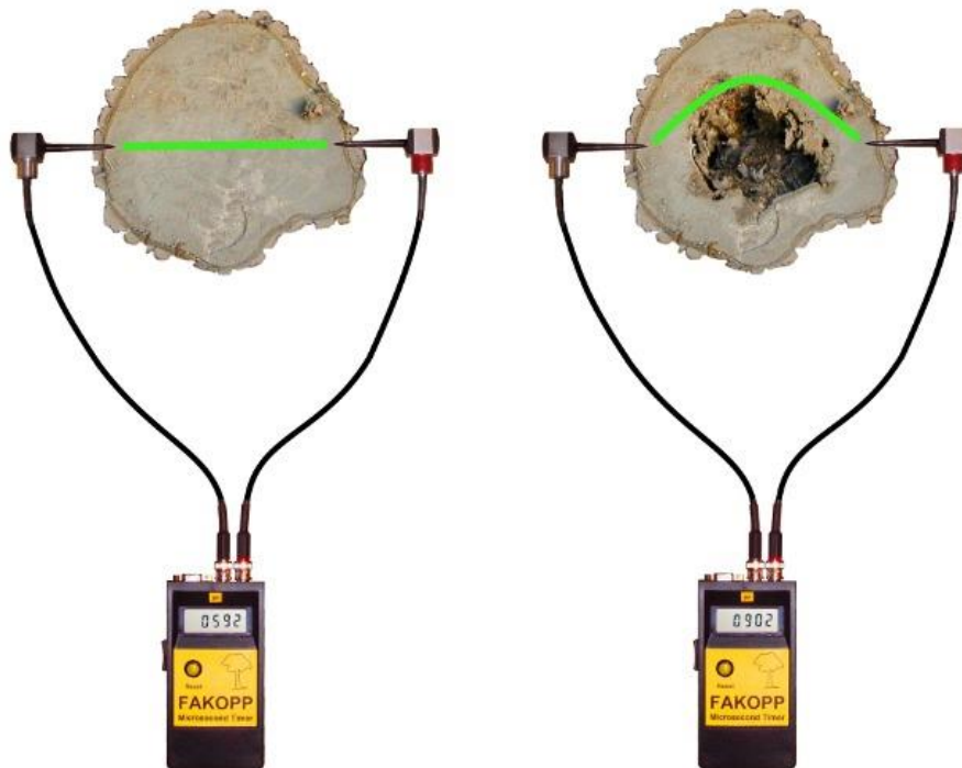
Figure 4 – Schematic photo showing the operation principle of the Microsecond Timer (Divos et al 2011)
