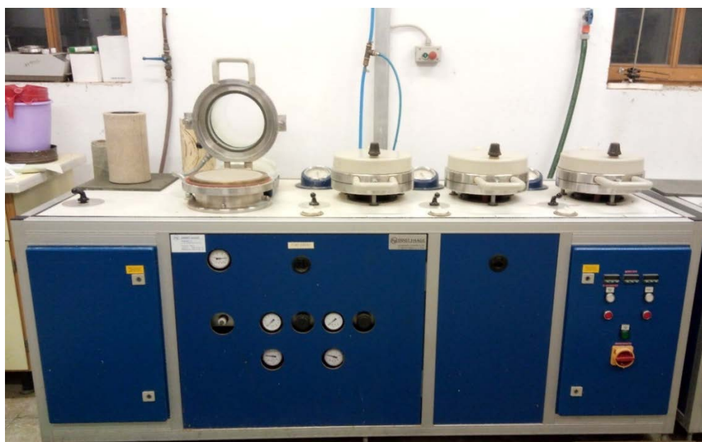
Figure 2.4 Photograph of laboratory sheet former with vacuum press-drying
