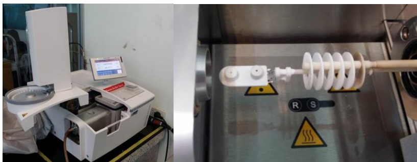
Figure 2.7 TGA instrument (left) and reference and sample pans were on a sensitive microbalance (right)
