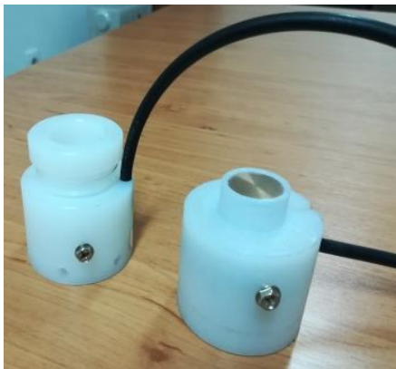
Figure 2.8 Photo of the home-made cell (Sopron University) used in photo-electrical characterizations of the films
