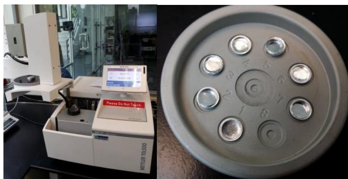
Figure 2.6 DSC instrument (left) and aluminum sample pans (40 \mu L) covered with the lids (right)
