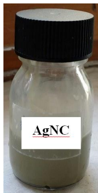
Figure 2.4 Silver nanocubes (AgNC) synthesized by polyol process
