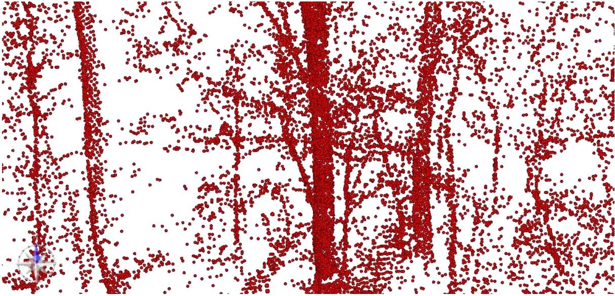
Figure 2-17. Stem surface points with significant amount of data reflected from other vegetation components. (Source data: Pro Silva demonstration site, Pilis, Hungary, 2006. Figure compiled by the author.)
