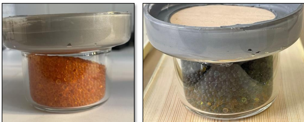
Figure 2.4 Silica gel in a cup before and after water absorption
