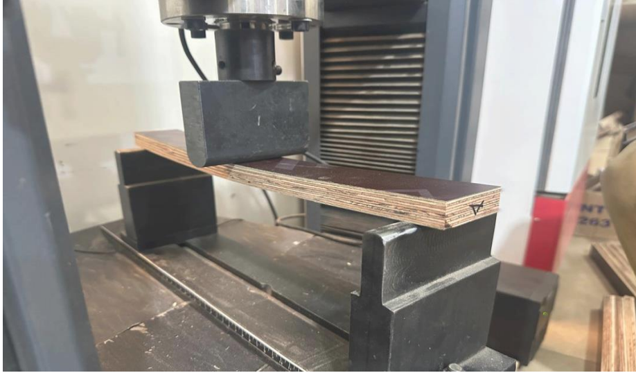
Figure 5: Plywood sample undergoing a 3-point bending test (Hegewald & Peschke UTM)
