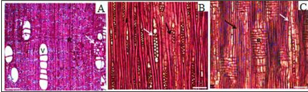
Figure 1.11 The higher the wood density is, the smaller the number of voids in the wood is and vice versa (A, C) Cross-sections of the Hevea brasiliensis wood. Scale bars:100 \mu\text{m} (Faria et al., 2021).
