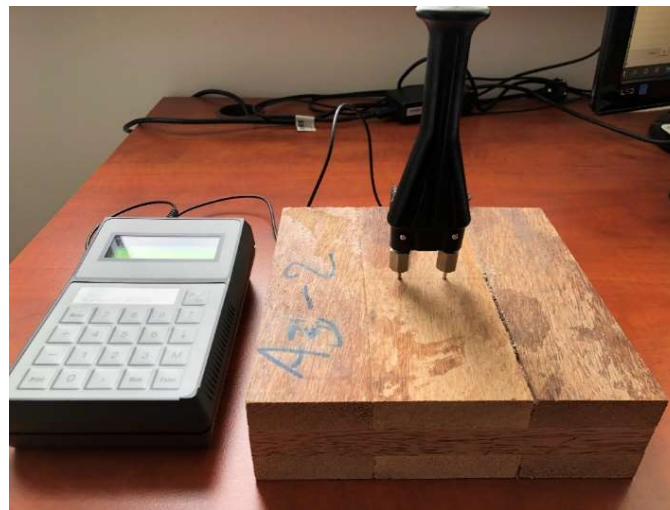
Figure 2.8 Photograph of testing the moisture content percentage of CTCP specimen.
