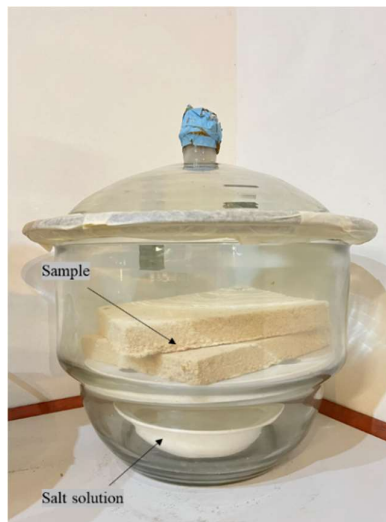
Figure 2.7 Photograph of water absorption test using a desiccator.
