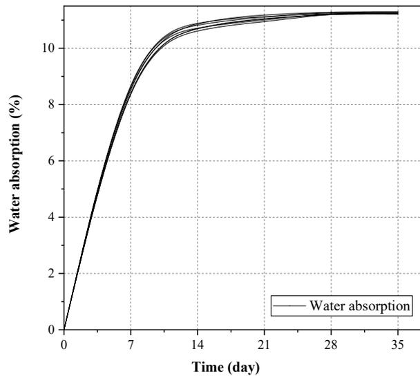
**Figure 1.** Water absorption percentages of bagasse fiberboard regarding the absorbent time.
