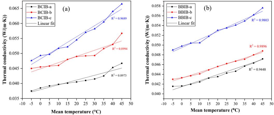
**Figure 3.** (a) Thermal conductivity of BCIB regarding the increase of mean temperatures; (b) Thermal conductivity of BBIB regarding the increase of mean temperatures.
