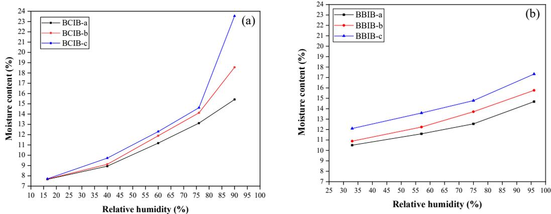
**Figure 2.** (a) Moisture content of BCIB regarding the increase of relative humidity levels; (b) Moisture content of BBIB regarding the increase of relative humidity levels.
