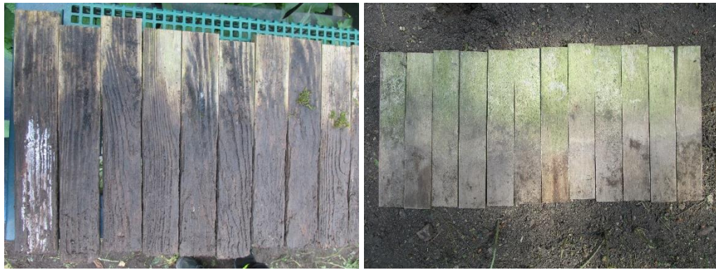
Figure A84. Severely damaged Scots pine stakes after 3.5 years (left), and sound acetylated hornbeam stakes after 4 years of exposure.
