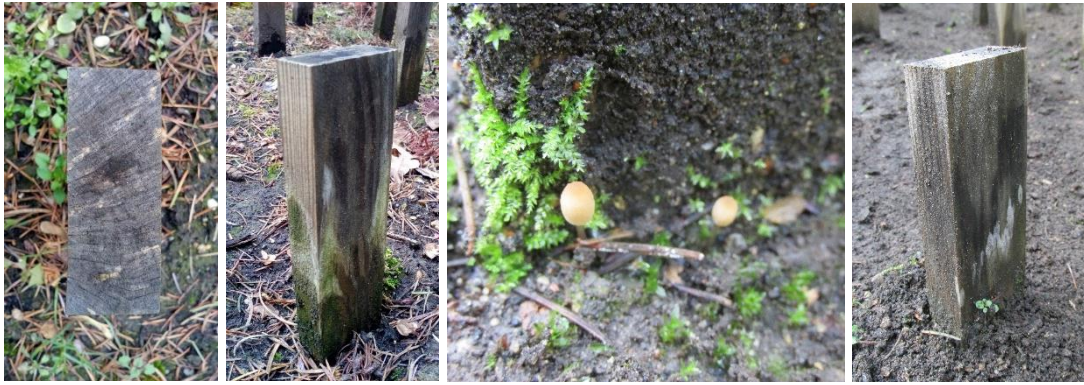
Figure A78. Wood degradation during exposure from left to right: wasp stripping (untreated hornbeam no.1, 11 months), algae (untreated Scots pine stake no.1, 11 months), mushroom of Coprinellus micaceus (untreated hornbeam stake no.12, 5 months), mycelium (untreated Scots pine stake no.1, 5 months).
