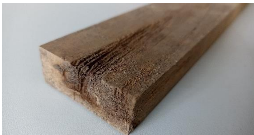
Figure 24. Acetylated hornbeam stake no. 7 which was taken from the test in order to examine its damage after 5.5 years.
