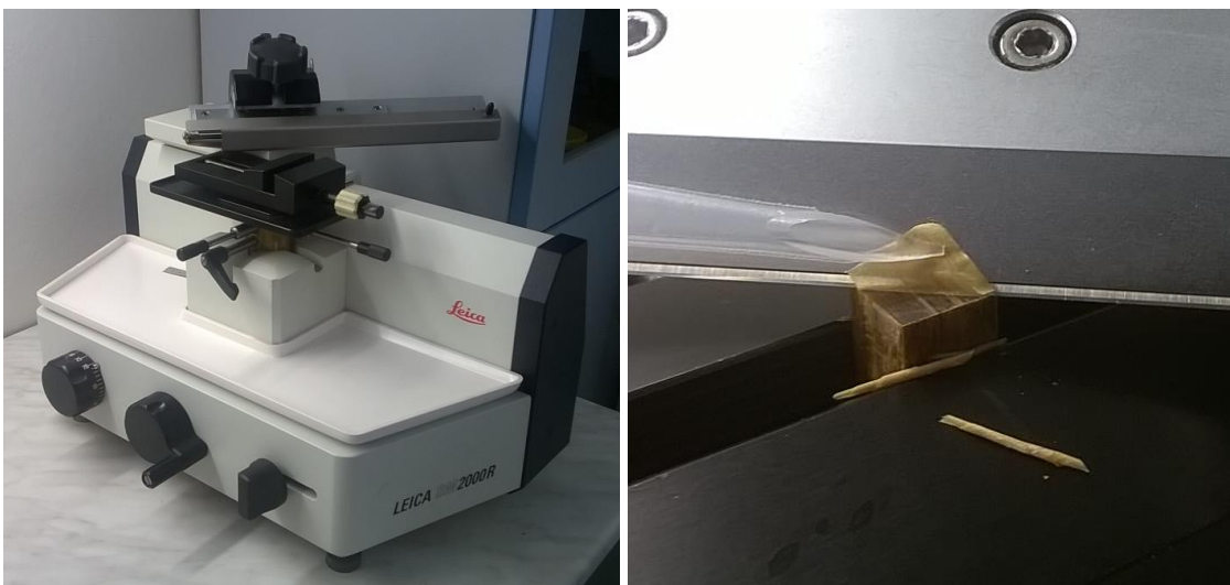
Figure A74. Microtome (left) and section cutting of acetylated wood (right).
