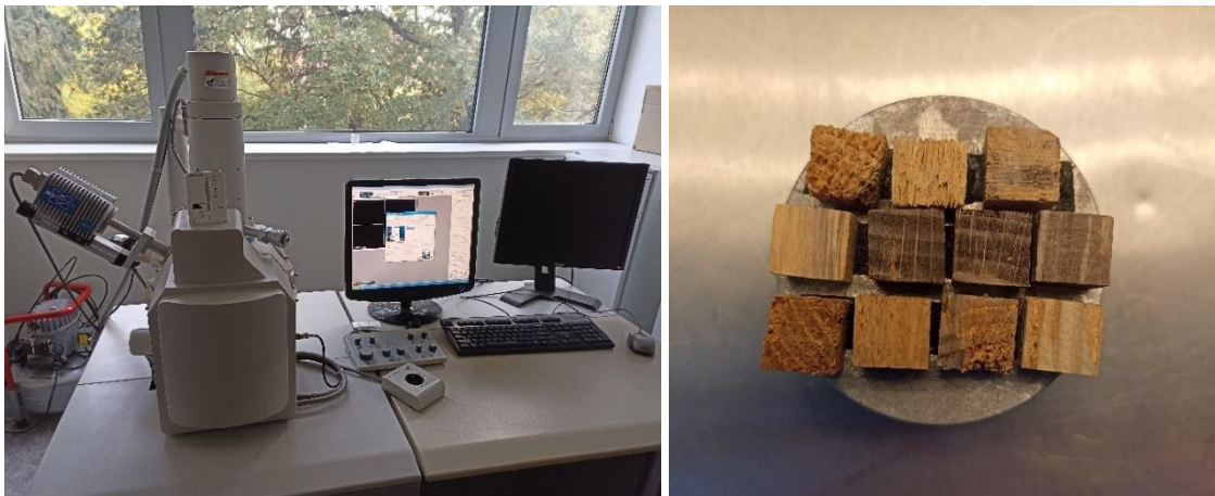
Figure A76. Hitachi S-3400N Scanning Electron Microscope (left) and samples on stage (right).
