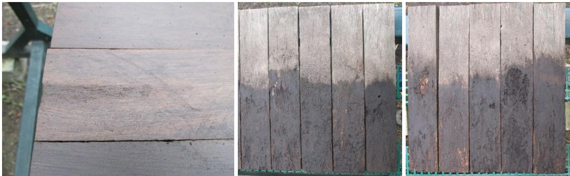
Figure A82. Brown rot in acetylated hornbeam stake no. 7 (left), decayed and insect-damaged untreated hornbeam (middle) and beech stakes (right) after 1.5 years of exposure.
