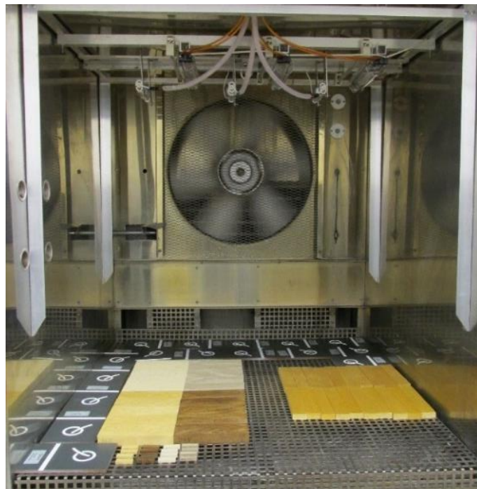
Figure 33. Uncoated and coated hornbeam and acetylated hornbeam samples placed in the ageing machine with mercury-vapor lamps.
