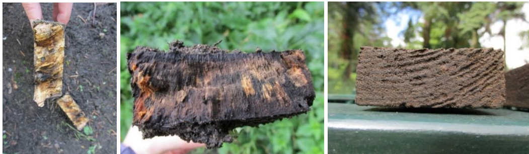
Figure A80. Failed untreated stakes from left to right: hornbeam stake no.3, beech stake no.6, and Scots pine stake no.1. after 6 months of exposure.
