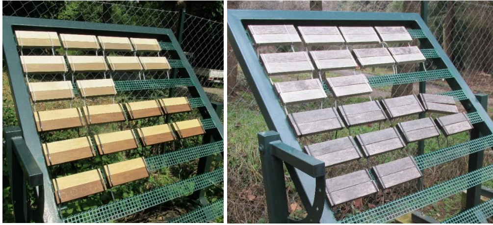
Figure 32. Uncoated and coated hornbeam and acetylated hornbeam samples exposed to weather on metal stand in Outdoor Exposure Testing Field. The photos were taken before (left, July 2016) and after weathering test (right, January 2018).
