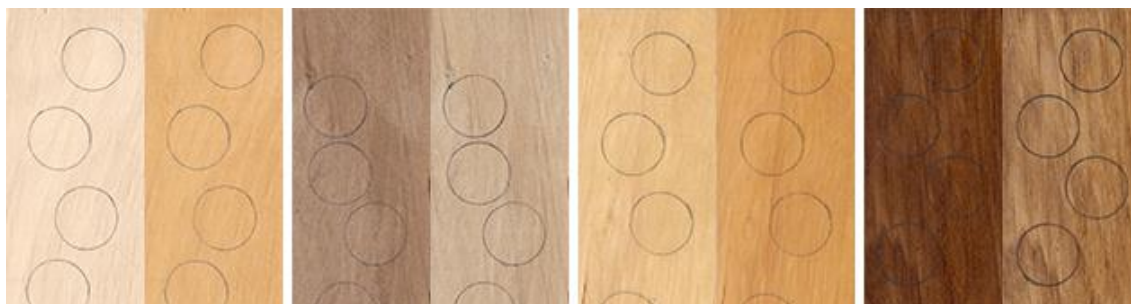
Figure 40. Scanned photos of hornbeam samples before and after being exposed to 200-hour-long mercury-vapor lamp irradiation. From left to right: untreated hornbeam, acetylated hornbeam, coated hornbeam, and coated and acetylated hornbeam.
