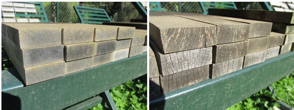
Figure A79. Sound acetylated hornbeam stakes (left) and untreated hornbeam stakes with wasp stripping, cracks, graying (right) after one year.
