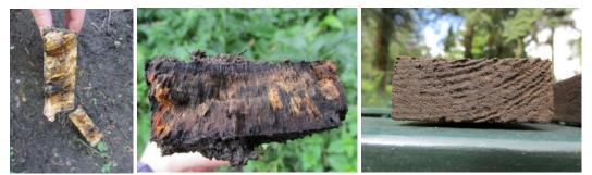
Figure A80. Failed untreated stakes from left to right: hornbeam stake no.3, beech stake no.6, and Scots pine stake no.1. after 6 months of exposure.
