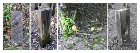
Figure A78. Wood degradation during exposure from left to right: wasp stripping (untreated hornbeam no.1, 11 months), algae (untreated Scots pine stake no.1, 11 months), mushroom of Coprinellus micaceus (untreated hornbeam stake no.12, 5 months), mycelium (untreated Scots pine stake no.1, 5 months).
