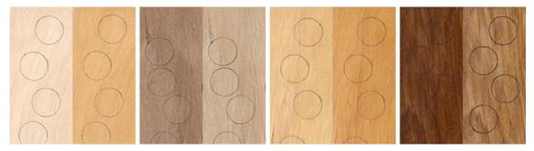
Figure 40. Scanned photos of hornbeam samples before and after being exposed to 200hour-long mercury-vapor lamp irradiation. From left to right: untreated hornbeam, acetylated hornbeam, coated hornbeam, and coated and acetylated hornbeam.
