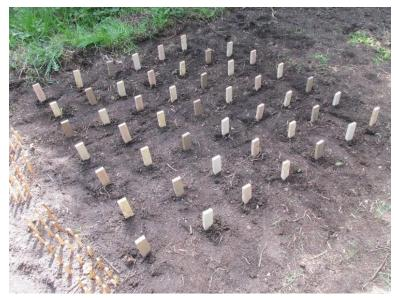
Figure 23. Stakes placed in soil in April 2016 in the outdoor exposure testing field. Twelve pieces of acetylated hornbeam, untreated hornbeam, beech and Scots pine stakes were buried half of their length.
