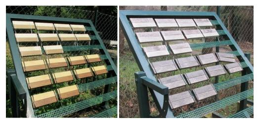
Figure 32. Uncoated and coated hornbeam and acetylated hornbeam samples exposed to weather on metal stand in Outdoor Exposure Testing Field. The photos were taken before (left, July 2016) and after weathering test (right, January 2018).
