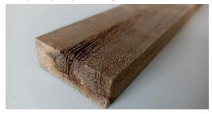
Figure 24. Acetylated hornbeam stake no. 7 which was taken from the test in order to examine its damage after 5.5 years.
