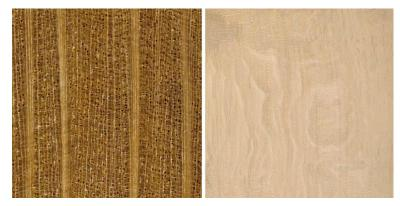
*Figure 7. Transverse section (left, ca. 10x) and radial section (right) of natural hornbeam wood (Richter and Dallwitz, 2019).*
