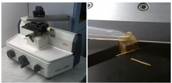
Figure A74. Microtome (left) and section cutting of acetylated wood (right).
