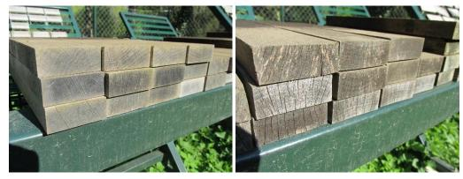
Figure A79. Sound acetylated hornbeam stakes (left) and untreated hornbeam stakes with wasp stripping, cracks, graying (right) after one year.
