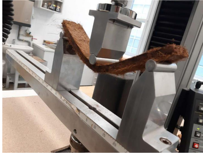
Figure 1.19: A flexural testing design for natural fiber reinforced composites using Instron universal testing equipment.
