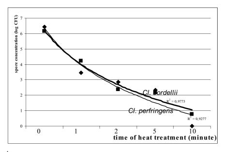
2<sup>nd</sup> figure: Curve calculated according to heat-resistance of *Cl. Perfringens* spores and *Cl. Sordellii* spores
