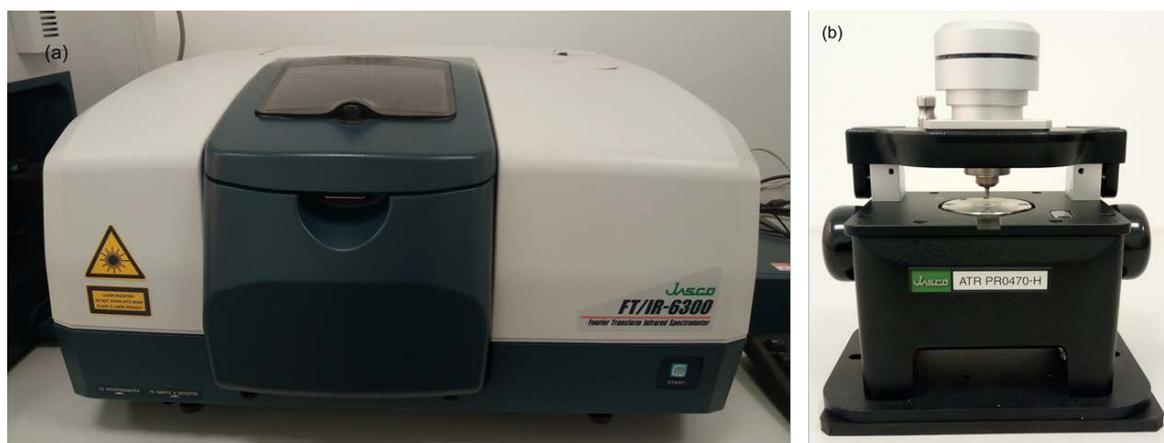
**Figure 2.8** Photographs of (a) FTIR and (b) ATR probe
