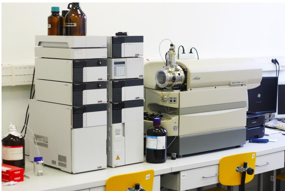
**Figure 2.6** Photograph of HPLC-DAD-MS/MS
