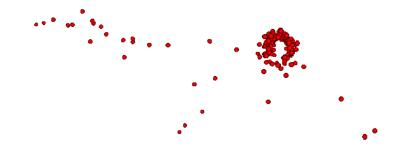
Figure 2-19. Stem surface points from multiple scanning positions in a 10 cm thick horizontal point cloud section. Isolated points have been reflected from probably branches. (Source data: Hidegvíz-völgy Forest Reserve, Hungary, 2006. Figure compiled by the author.)
