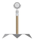
Figure 2-7. Target object for registration of scans. (www.riegl.com)
