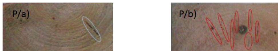
(a) Lack of end checking in the sample exposed to moderate IR radiation. The blue ring indicates a material failure spotted already before the IR treatment. According to the connecting temperature profile of Fig. 6.6a., the maximum temperature difference between the core and the surface was 25 °C
