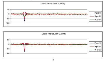
R profile it's questioned if the R profile derived from the traditional gauss filter is suitable for the quantitative evaluation of big porous species. The distortion of R profile is caused by the waviness filtration. Needs to be investigated the necessity of filtering and the interlocution possibility of the traditional Gauss filter.
