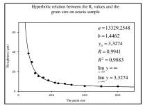
and  $R_z$  showed  $y = y_o + \frac{a}{r^n}$ hyperbolic dependence from the grain size. This way by vessel removal the expected relation was obtained between Pz, Rz and the grain size. The limit roughness of the investigated samples was around 5 µm for P<sub>z</sub> and about 3-4 um for  $R_z$ . Based upon the  $P_z/R_z$ relation investigations
